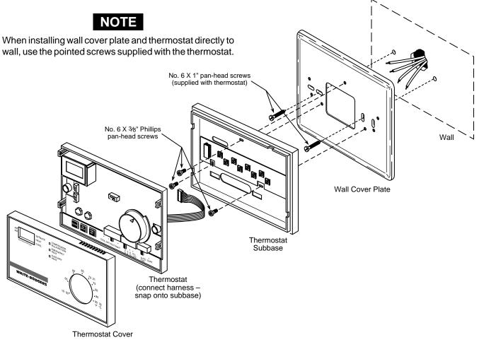
Figure 12. Mounting 1F62 thermostat to wall
